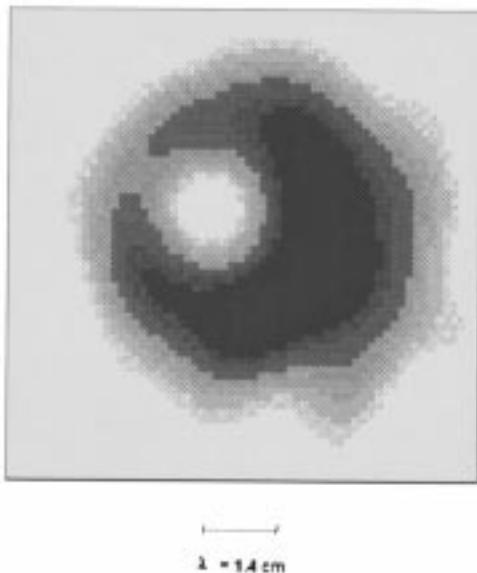
Fig. 7. Reconstruction after five iteration of the real part of the permittivity of the liquid phantom (two asymmetrically in closed container) place in water.
