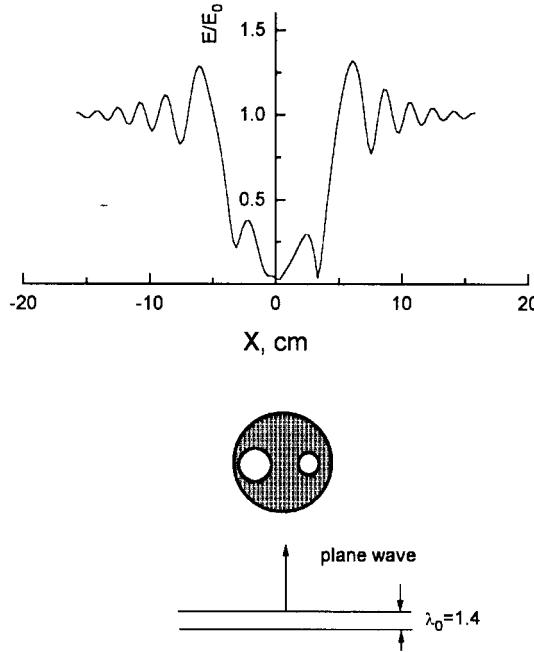
Fig. 1. Diffraction of a plane wave on the model object with the permittivity of the myocardium tissue surrounded by the water.
