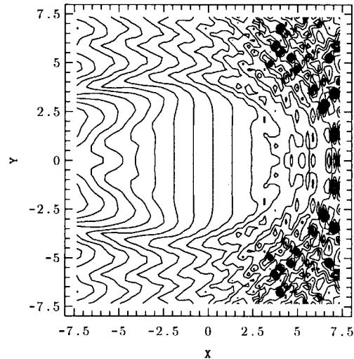
Fig. 2. Generation of plane wave by 32 transmitters.
