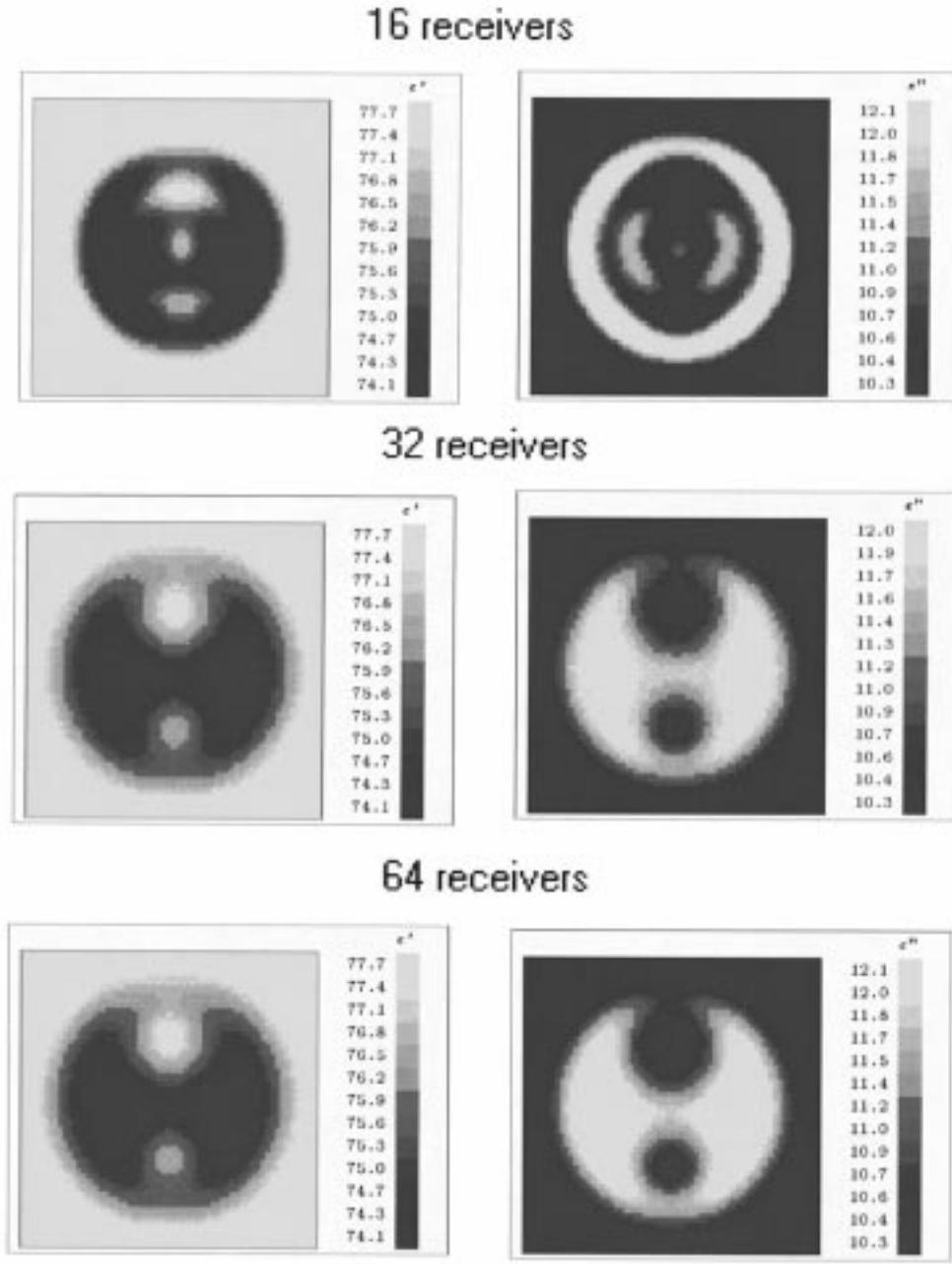
Fig. 3. Comparison of the object reconstruction with different numbers of receivers.
